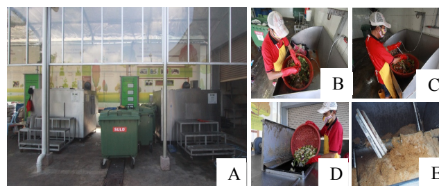
Figure 3 (A) Two units of Bio-mate food waste composting machine at Sutera Mall's Good Earth Center. Capacity of each unit is 250 kg food waste/day. Steps for processing the food waste include: (B) sorting out inorganic waste, (C) pre-rinse with water, (D) loading into the machine, and (E) adding sawdust into the mix.
